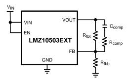
Figure 22. Loop Compensation Control Components
