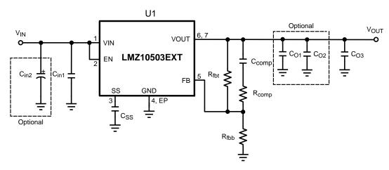
Figure 26. Schematic for 2.5-V Output Based on 3.3-V to 5-V Input
