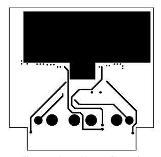
Figure 32. Internal Layer 1 (Ground)
