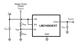
Figure 18. Tracking Using External Power Supply
