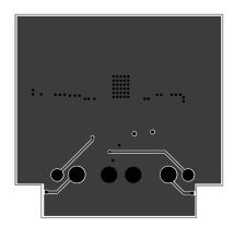
Figure 33. Internal Layer 2 (Ground and Signal Traces)
