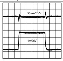
$$100~\mu s/DIV$$   $V_{IN}$  = 5.0 V,  $V_{OUT}$  = 2.5 V,  $I_{OUT}$  = 0.3-A to 2.7-A to 0.3-A step 20-MHz Bandwidth Limited
