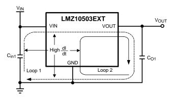
Figure 29. Critical Current Loops to Minimize
