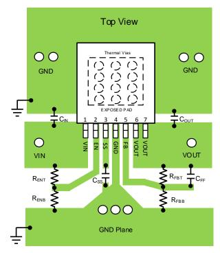
Figure 30. PCB Layout Guide
