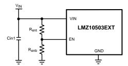
Figure 16. Setting Enable and UVLO
