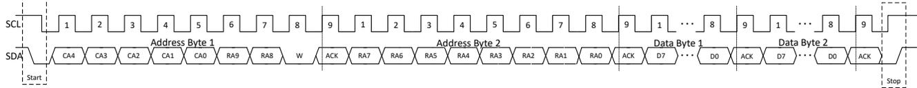
**Figure 8-14. I<sup>2</sup>C Write Timing**
