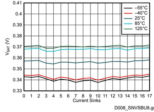
**Figure 7-6.  $V_{SAT}$  vs Current Sinks (50 mA)**
