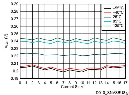
**Figure 7-8.  $V_{SAT}$  vs Current Sinks (10 mA)**
