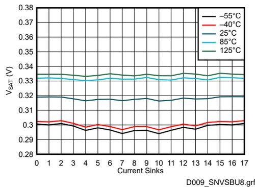
**Figure 7-7.  $V_{SAT}$  vs Current Sinks (30 mA)**
