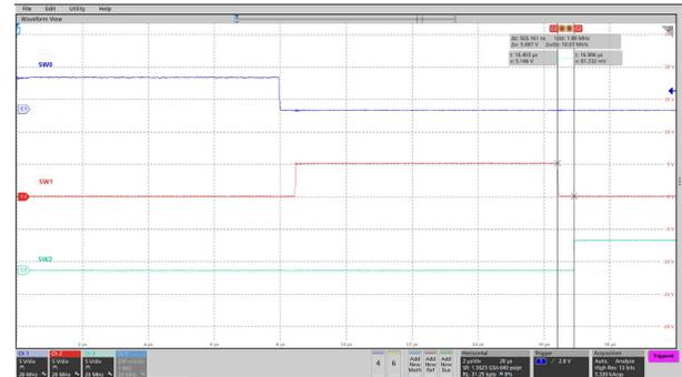
Switch blank time  $t_{SW\_BLK} = 0.5 \mu s$
