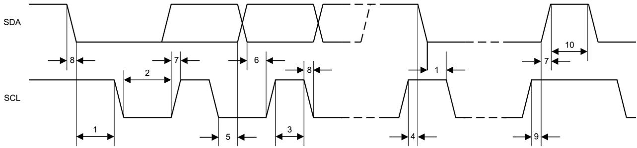
**Figure 7-2. I<sup>2</sup>C Timing Parameters**
