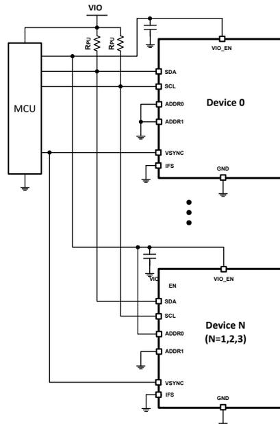
**Figure 8-16. I<sup>2</sup>C Multiple Devices Connection**
