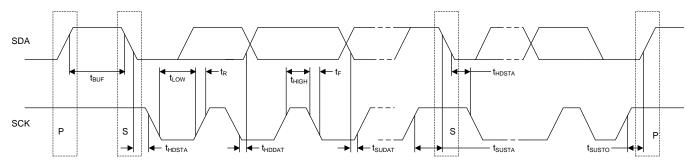
Figure 14. I<sup>2</sup>C Timing Diagram
