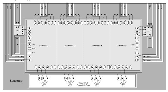
Figure 42. Basic Application Circuit with Pad Control
