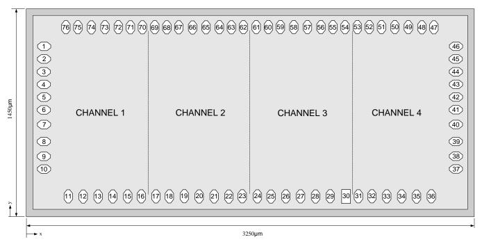
Figure 46. Chip Dimensions and Pad Locations
