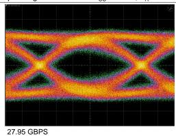
Figure 10. Output Eye-Diagram, 30 μA<sub>P-P</sub> Input Current
