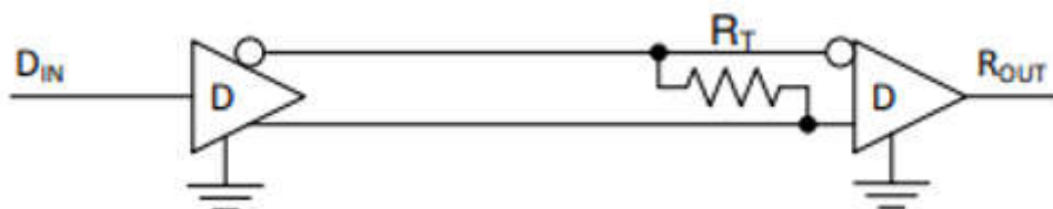
Figure 8-1. Typical RS-485 or RS-422 Application with Terminated Receiver.
