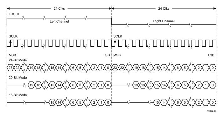
Figure 25. Right Justified 48-f<sub>S</sub> Format
