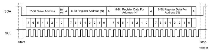
Figure 27. Typical I<sup>2</sup>C Sequence
