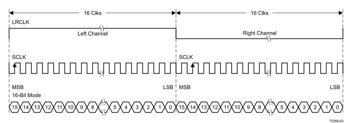
Figure 26. Right Justified 32-f<sub>S</sub> Format
