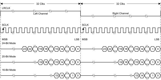
Figure 24. Right Justified 64-f<sub>S</sub> Format
