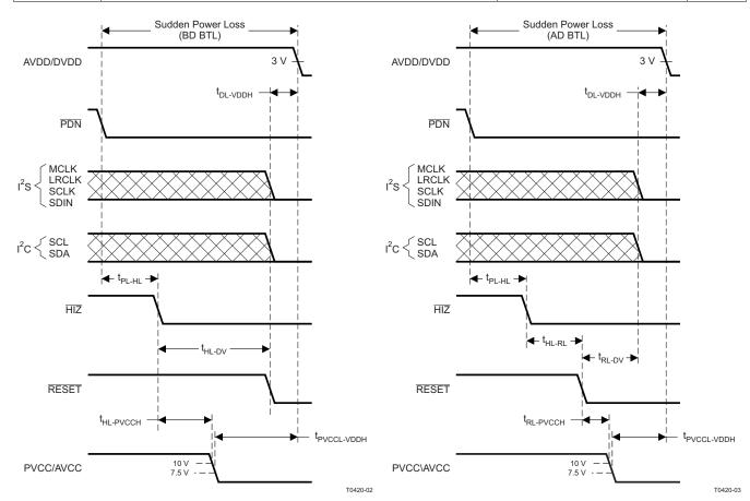
Figure 39. BD BTL Power Loss Sequence
