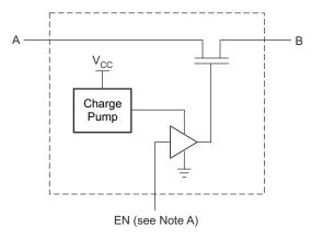
Note A: EN is the internal enable signal applied to the switch.
