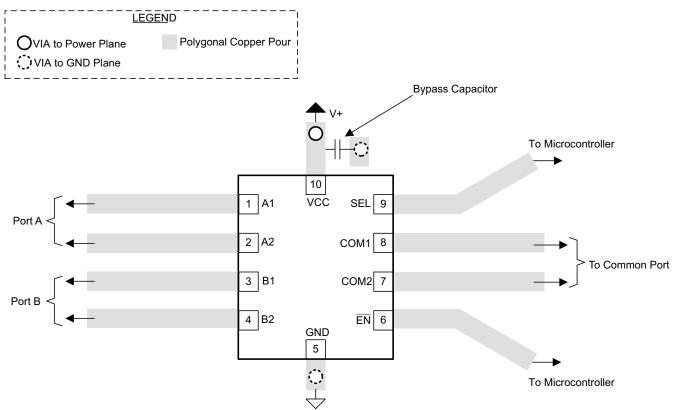
Figure 9-19. Package Layout Diagram
