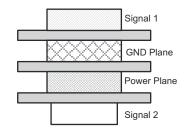
Figure 9-18. Four-Layer Board Stack-Up
