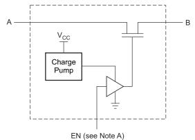
Note A: EN is the internal enable signal applied to the switch. Functional Block Diagram
