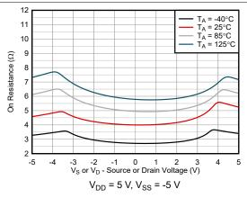
Figure 5-6. On-Resistance vs Temperature
