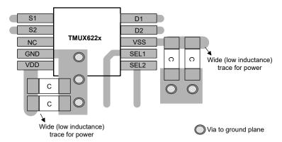
Figure 8-4. TMUX622x Layout Example
