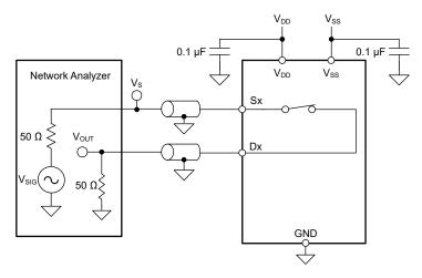
Figure 6-10. Bandwidth Measurement Setup
