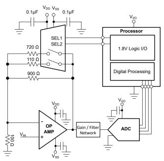
Figure 8-1. Gain Switching
