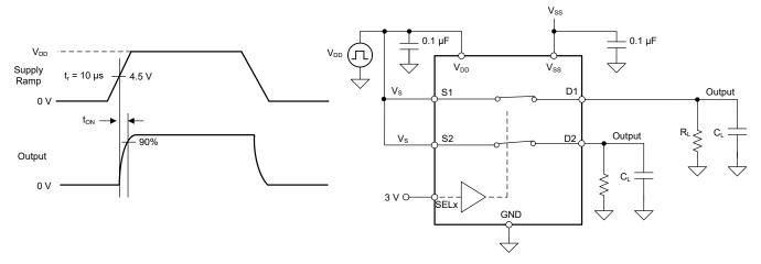
Figure 6-5. t<sub>ON (VDD)</sub> Time Measurement Setup
