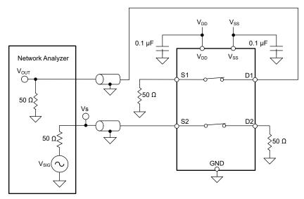
Figure 6-9. Crosstalk Measurement Setup
