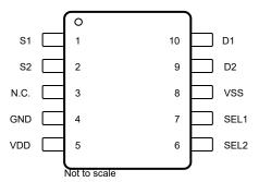
Figure 4-1. DGS Package, 10-Pin VSSOP (Top View)
