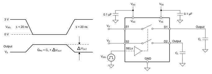
Figure 6-7. Charge-Injection Measurement Setup
