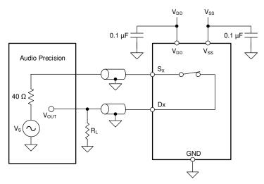
Figure 6-11. THD + N Measurement Setup
