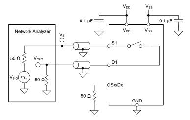
Figure 6-8. Off Isolation Measurement Setup
