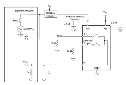
Figure 6-12. AC PSRR Measurement Setup
