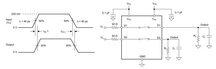
Figure 6-6. Propagation Delay Measurement Setup
