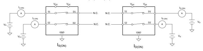
Figure 6-3. On-Leakage Measurement Setup
