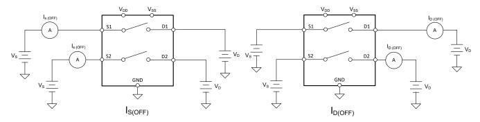
Figure 6-2. Off-Leakage Measurement Setup
