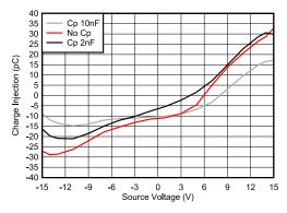
Figure 7-2. Charge Injection Compensation
