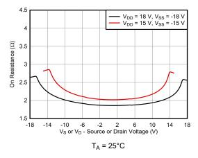
Figure 8-2. On-Resistance vs Source or Drain Voltage
