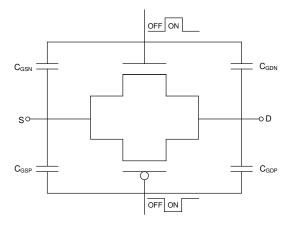
Figure 7-1. Transmission Gate Topology
