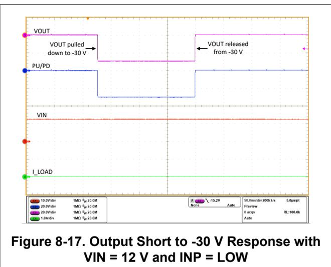
Figure 8-17. Output Short to -30 V Response with VIN = 12 V and INP = LOW
