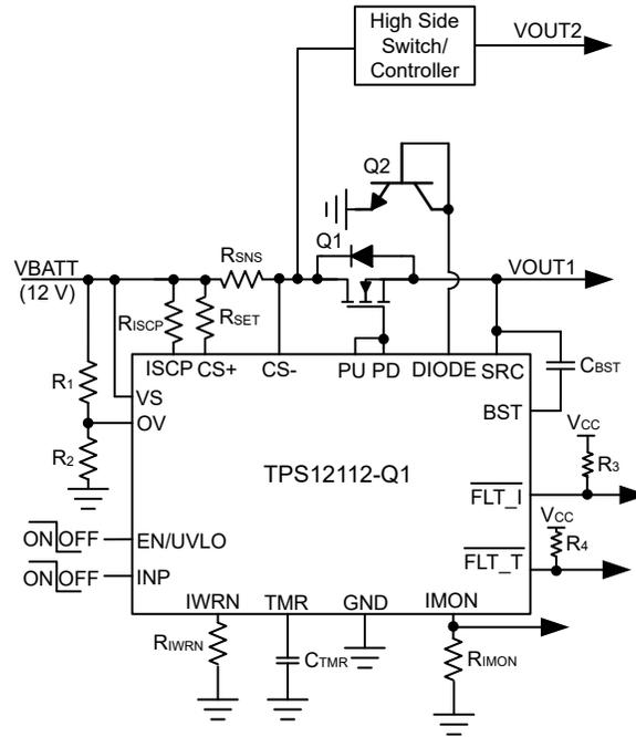
Figure 8-13. TPS12112-Q1 Application Circuit with Grouped IMON Output
