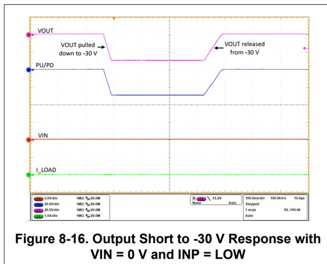
Figure 8-16. Output Short to -30 V Response with VIN = 0 V and INP = LOW
