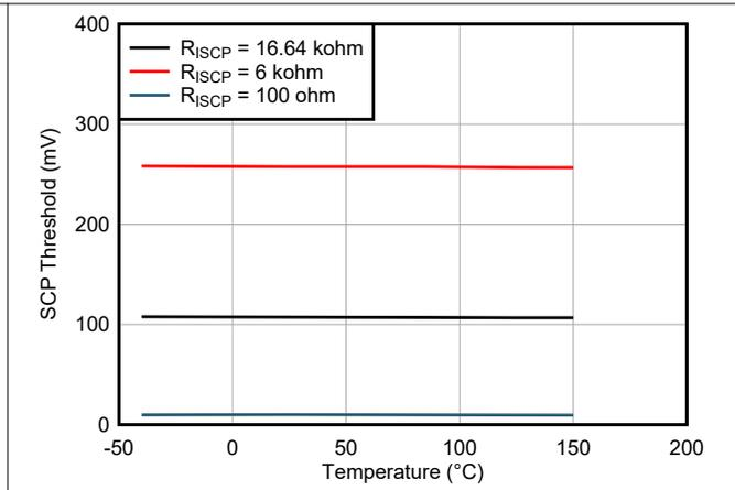
Figure 6-8. Short-Circuit Threshold ( $V_{(SNS\_SCP)}$ ) vs Temperature
