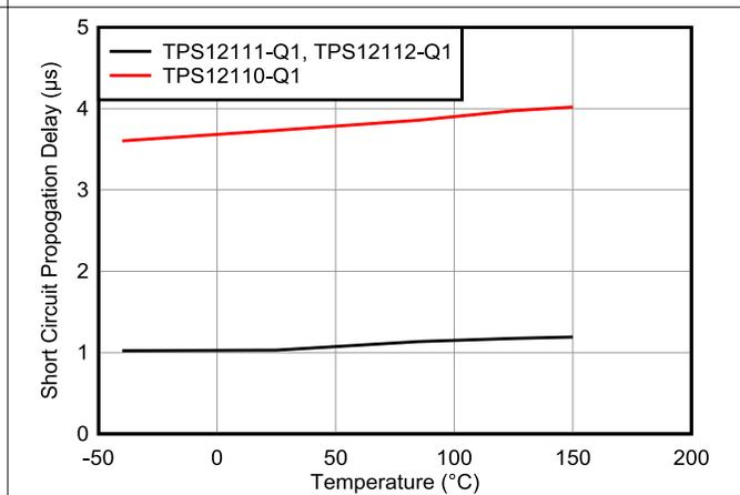
Figure 6-12. Short Circuit Protection Response Time ( $t_{sc}$ ) vs Temperature
