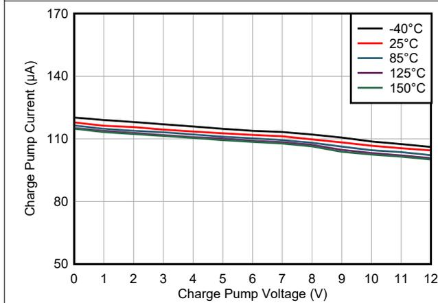
Figure 6-3. Charge Pump Current vs Charge Pump Voltage
