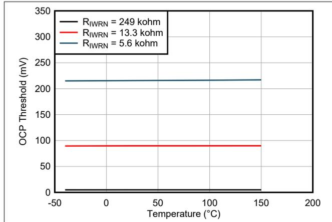
Figure 6-7. Overcurrent Threshold ( $V_{(SNS\_WRN)}$ ) vs Temperature
