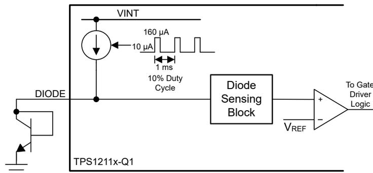
Figure 8-15. DIODE based Remote Temperature Sensing Block Diagram
