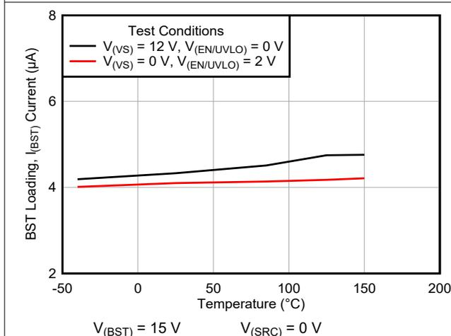
Figure 6-5. BST Loading Current ( $I_{BST}$ ) vs Temperature
