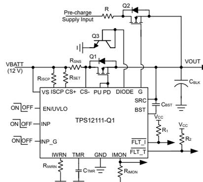
Circuit Breaker for DC/DC Converter
