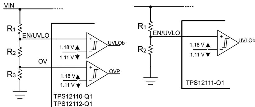
Figure 8-14. Programming Overvoltage and Undervoltage Protection Threshold
