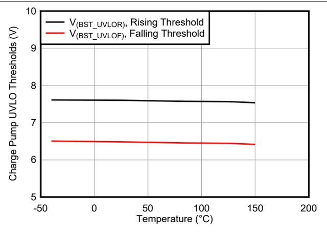
Figure 6-6. Charge Pump UVLO Thresholds vs Temperature
