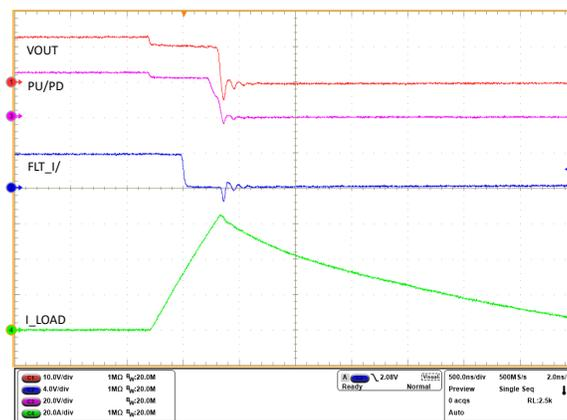
**Figure 9-12. Output Hot-Short Response of the TPS1211-Q1 Device**
