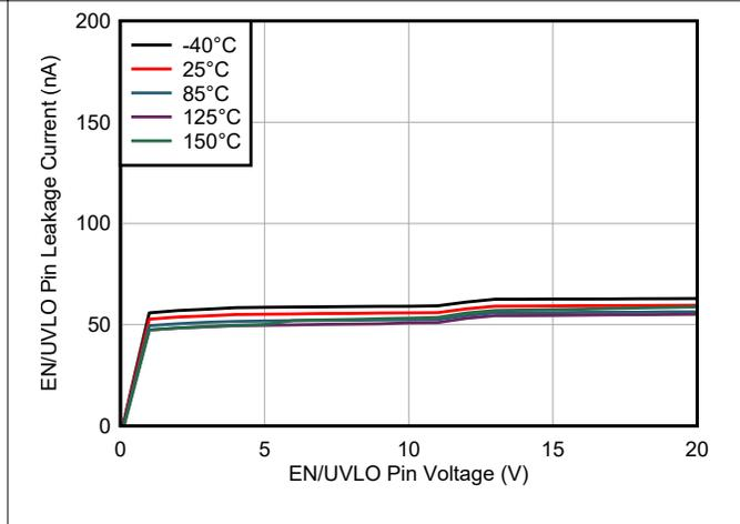
Figure 6-10. EN/UVLO Pin Voltage vs Leakage Current
