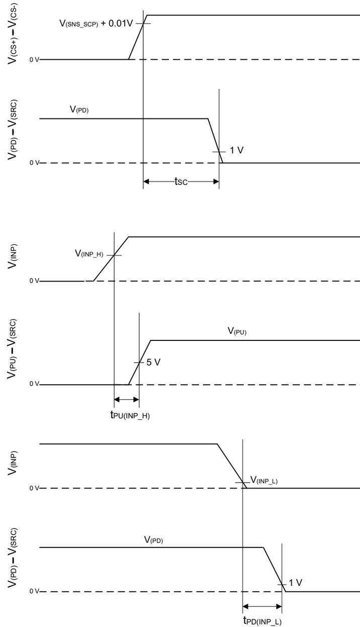
**Figure 7-1. Timing Waveforms**
