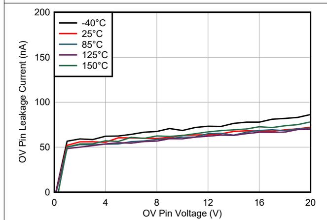
Figure 6-11. OV Pin Voltage vs Leakage Current
