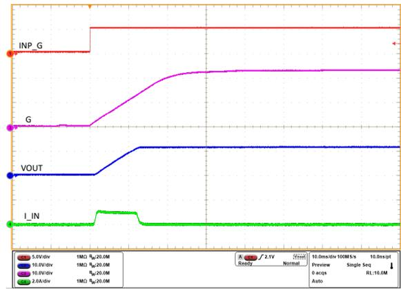
**Figure 9-11. Precharge Profile of the Output Capacitance (VIN = 12 V, C<sub>OUT</sub> = 1 mF, No Load)**
