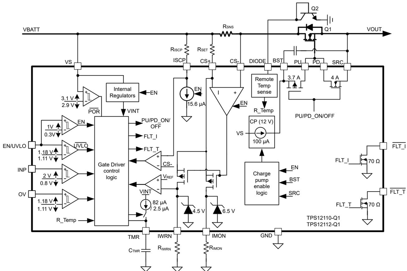
**Figure 8-1. TPS12110-Q1 and TPS12112-Q1 Functional Block Diagram**
