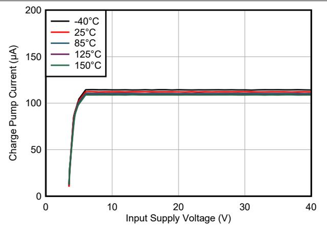
Figure 6-4. Charge Pump Current vs Input Supply Voltage
