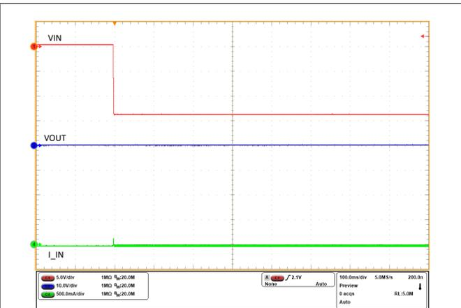
Figure 9-15. Input Reverse Polarity Protection with TPS12110-Q1
