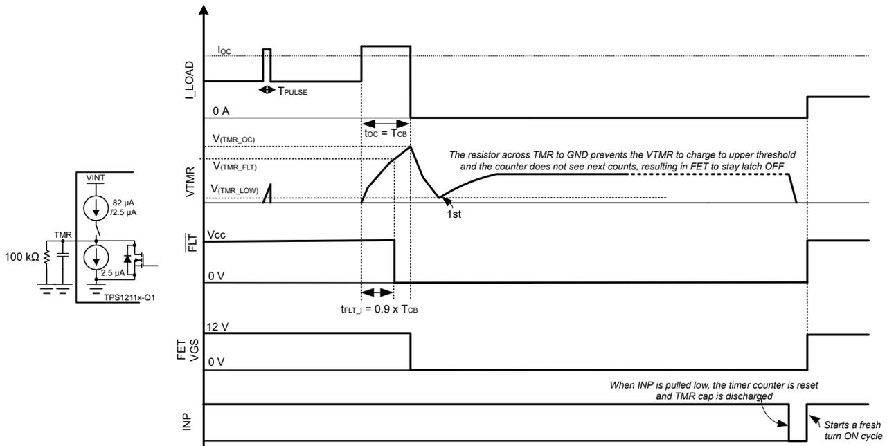
Figure 8-11. Overcurrent Protection with Latch-Off
