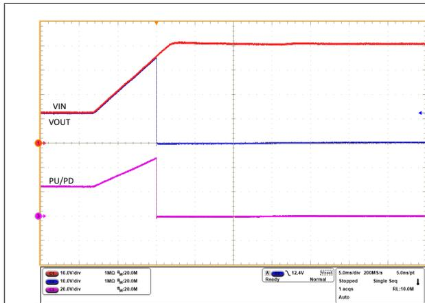
Figure 9-14. Overvoltage Cutoff Response of TPS12110-Q1 at 36-V Level
