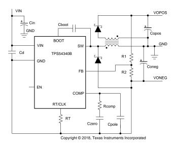
Figure 51. TPS54360B Split Rail Power Supply
