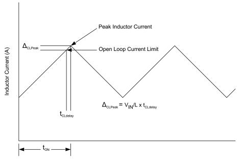
Figure 23. Current Limit Delay
