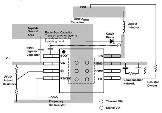
Figure 52. PCB Layout Example
