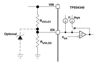
Figure 22. Adjustable Undervoltage Lockout (UVLO)
