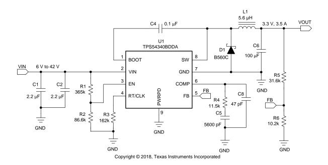
Figure 32. 3.3 V Output TPS54340B Design Example
