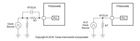
Figure 24. Synchronizing to a System Clock
