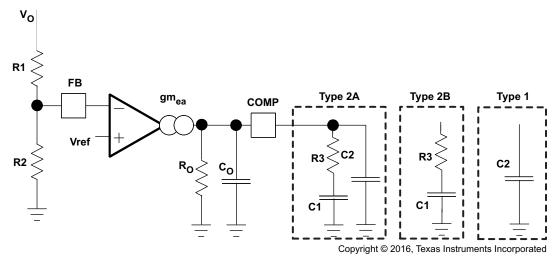
Figure 30. Types of Frequency Compensation
