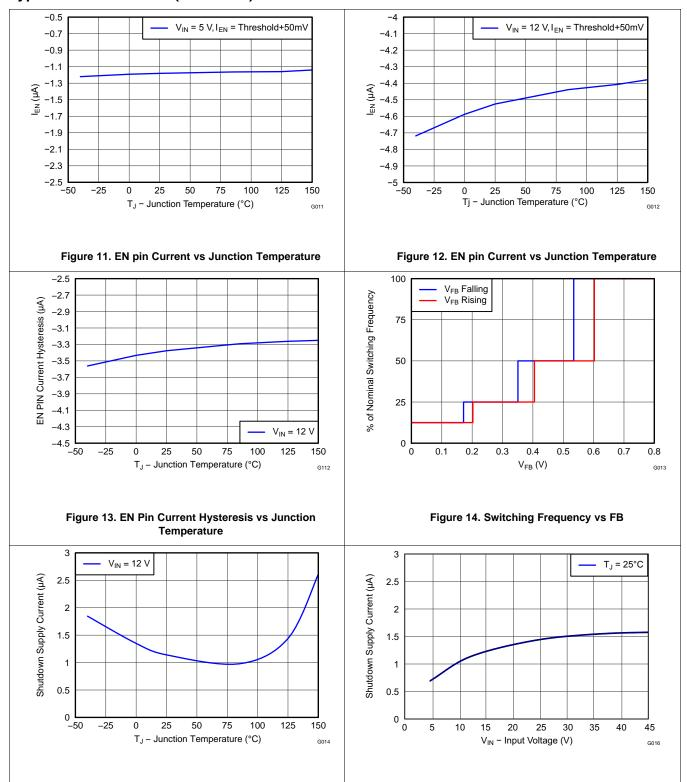
Figure 15. Shutdown Supply Current vs Junction Temperature
