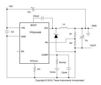
Figure 50. TPS54340B Inverting Power Supply
