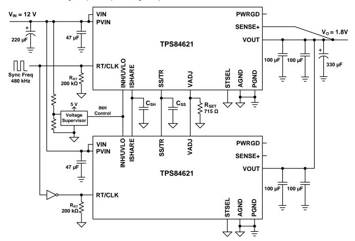
Figure 26. Typical TPS84621 Parallel Schematic
