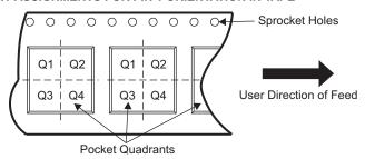
Reel Diameter Reel Width W1 Package Type Package Drawing A0 (mm) B0 (mm) K0 (mm) P1 (mm) W (mm) Pin1 Quadrant Device Pins (mm) (mm) TPS84621RUQR B1QFN RUQ 47 500 330.0 24.4 9.35 15.35 3.1 16.0 24.0 Q1 B1QFN TPS84621RUQT RUQ 47 250 330.0 24.4 9.35 15.35 3.1 16.0 24.0 Q1
