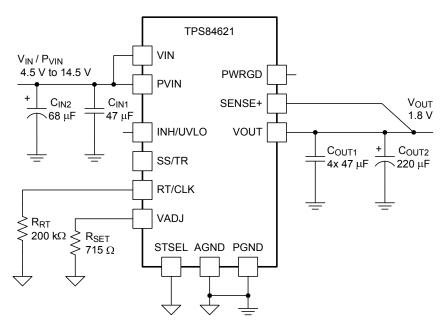
Figure 23. Typical Schematic PVIN = VIN = 4.5 V to 14.5 V, VOUT = 1.8 V
