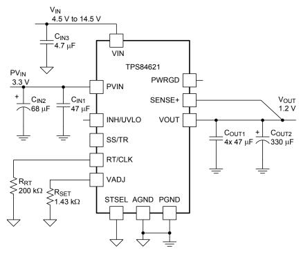
Figure 25. Typical Schematic PVIN = 3.3 V, VIN = 4.5 V to 14.5 V, VOUT = 1.2 V
