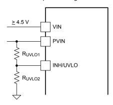
Figure 42. Adjustable PVIN Undervoltage Lockout, (VIN ≥4.5 V)
