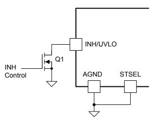
Figure 29. Typical Inhibit Control
