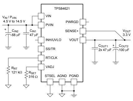
Figure 24. Typical Schematic PVIN = VIN = 4.5 V to 14.5 V, VOUT = 3.3 V
