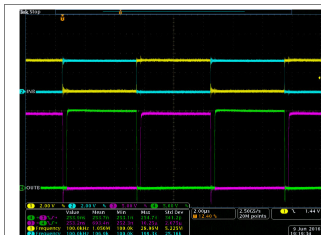
Figure 8-5. Bench Test Waveform for INA/B and OUTA/B
