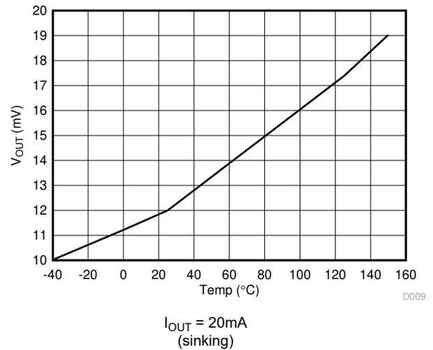
**Figure 6-11. V<sub>OL</sub> versus Temperature**
