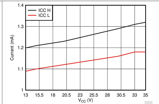
Figure 6-5. Supply current versus Supply Voltage
