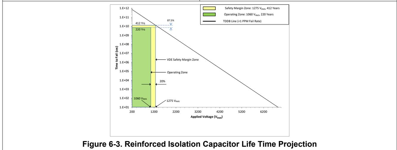
**Figure 6-3. Reinforced Isolation Capacitor Life Time Projection**
