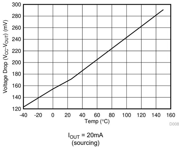
**Figure 6-10. V<sub>OH</sub> (20mA Load) versus Temperature**
