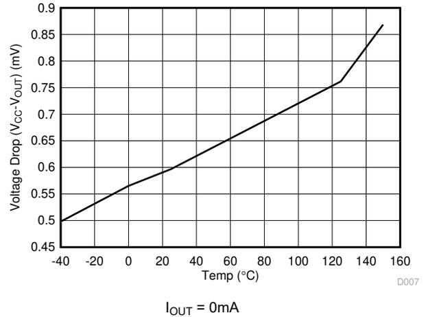
**Figure 6-9. V<sub>OH</sub> (No Load) versus Temperature**
