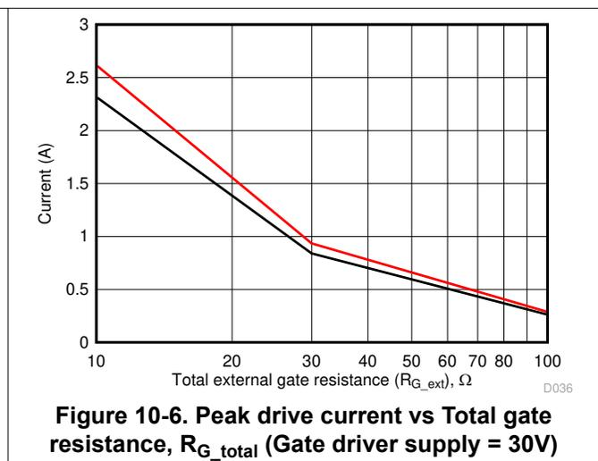
Use Table 10-3 to find the minimum gate resistance to be used with UCC23511-Q1 when driving a power switch. The values shown includes the power switch internal gate resistance  $R_{G\_int}$ . Hence,  $R_{G\_int}$  must be subtracted from the values shown to determine the value of the resistor to populate on the printed circuit board.
