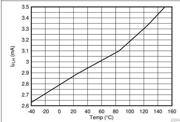
Figure 6-6. Forward threshold current versus Temperature
