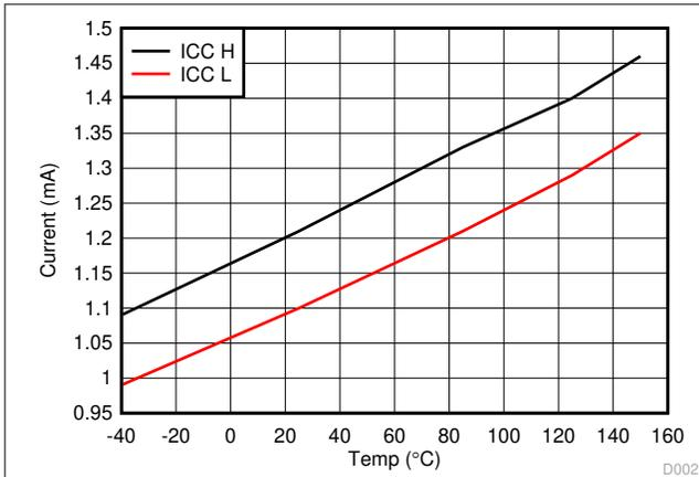
Figure 6-4. Supply currents versus Temperature
