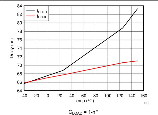
Figure 6-7. Propagation delay versus Temperature
