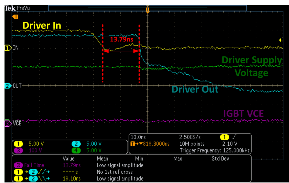
Figure 8-3. UCC27624-Q1 Used to Drive IGBT in the Boost Converter
