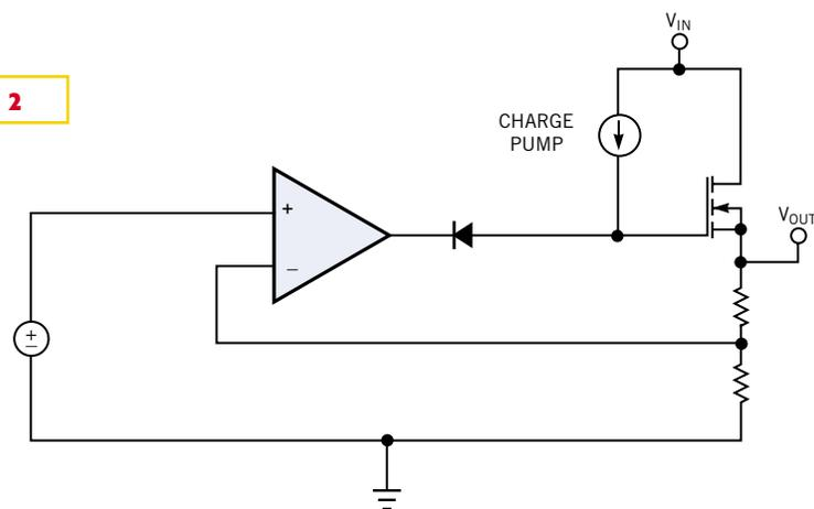
A previous approach to driving an n-type-DMOS pass element uses a charge pump to directly drive the gate, which leads to high noise and limited positive slew rate.
