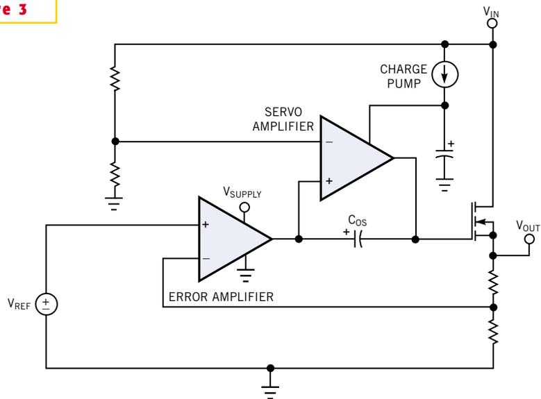
**A new topology uses a fast voltage-control amplifier to control the gate and a slow servo amplifier to maintain the proper offsetting voltage across a dc level-shift, or offsetting, capacitor,  $C_{OS}$ .**
