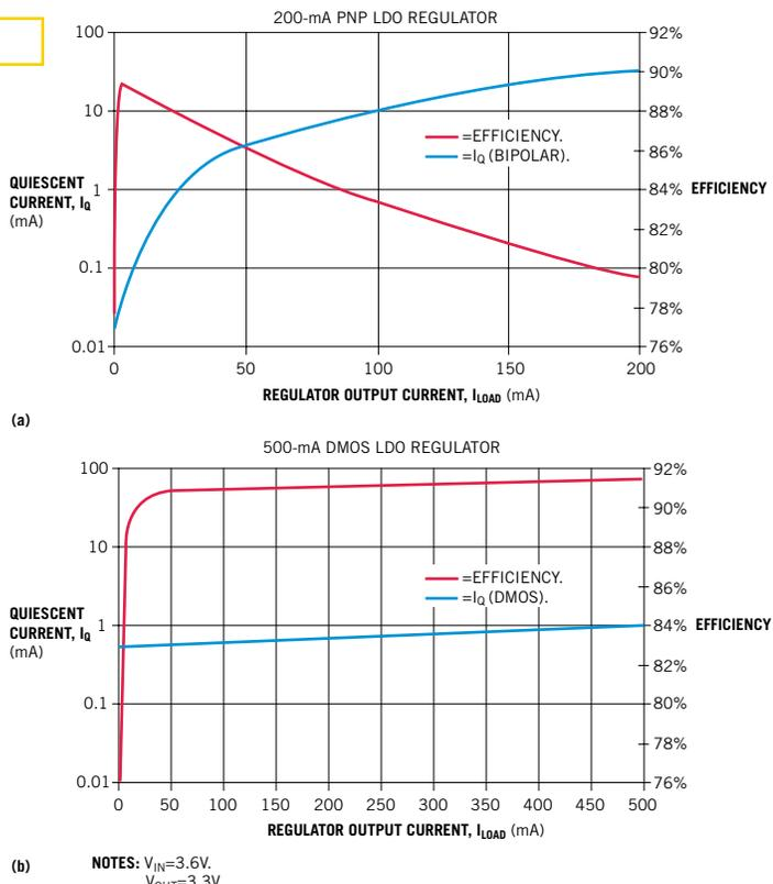
**Even a so-called micropower regulator with a pnp pass element and a featured quiescent current of 20  $\mu$ A can draw 30 mA, or 13% of its rated supply current, at its maximum rated load of 200 mA (a). A DMOS LDO regulator, the REG103, features a quiescent-current draw of 1 mA at the full-rated, 500-mA load (b).**
