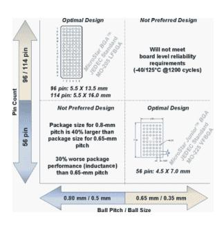
(thin scale small outline package) logic package. With a ball pitch of 0.65mm, the MicroStar Jr. TM offers a 30% performance (Inductance) improvement over 56-pin BGA with 0.8mm ball
