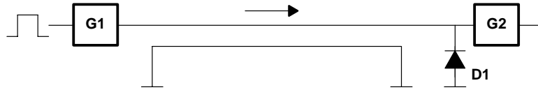
Figure 27. Typical Point-to-Point Connection
