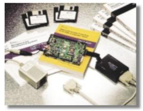
• C Compiler—it accepts ANSI C source code and produces efficient C2000 assembly language code. It is able to perform a variety of optimizations to improve the density and efficiency of the compiled code.
