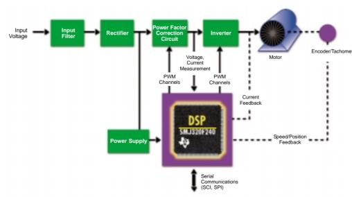
With a high level of peripheral integration and powerful computational abilities, the SMJ320F240 become the center of many different control applications.
