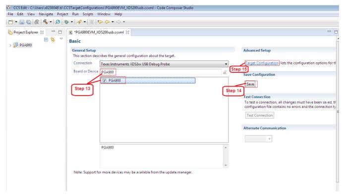
Figure 13. XDS200 Emulator Device Configuration
