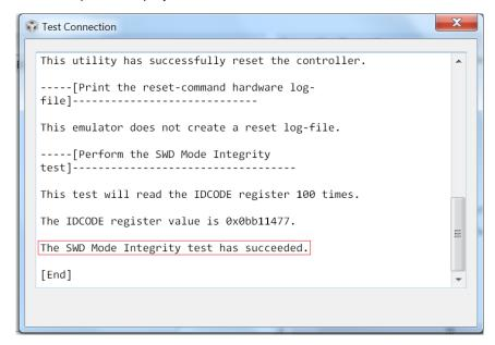
Figure 17. XDS200 USB Emulator Test Connection Report
