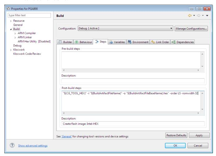
Figure 9. Flash Image Intel Hex Configuration
