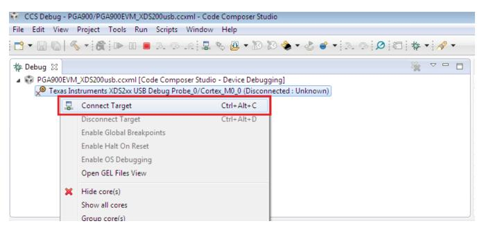
Figure 20. Connect to the PGA900EVM
