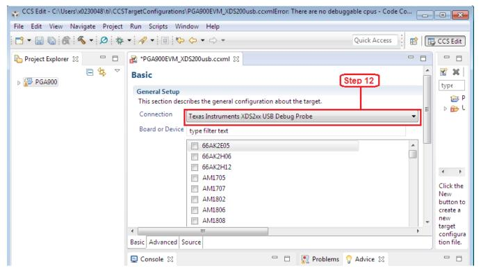
Figure 12. XDS200 Emulator Connection Configuration
