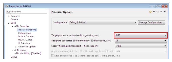
Figure 6. Target Processor Cortex M0 Selection
