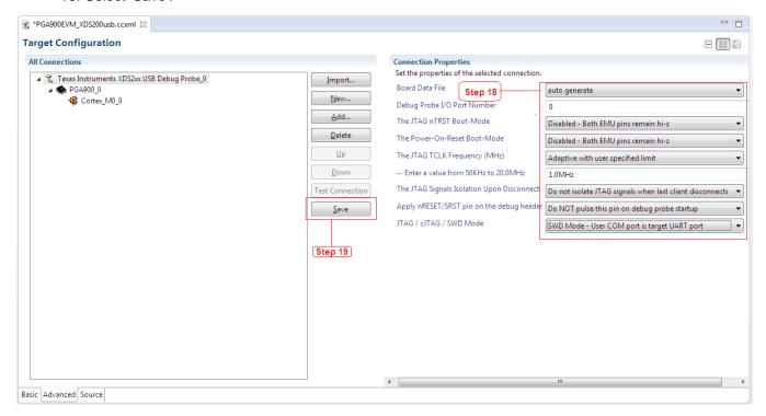
Figure 15. XDS200 USB Emulator Connection Properties
