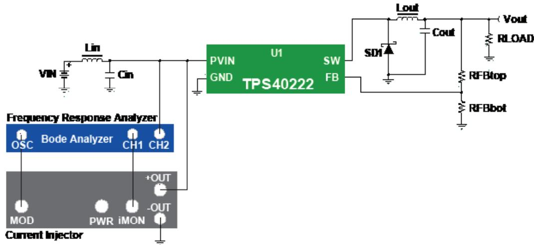
Figure 34 – Filter/converter impedance measurement setup.
