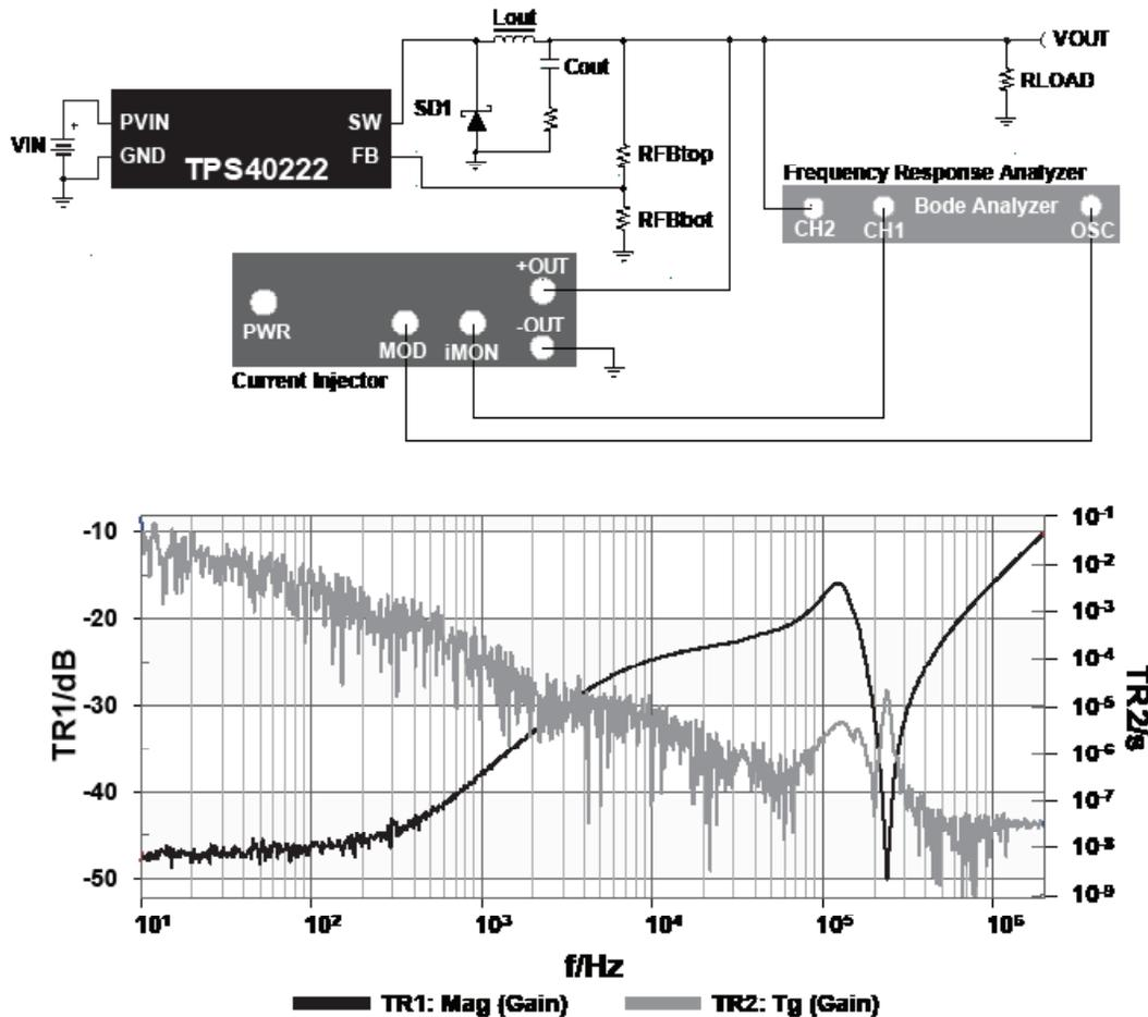
Figure 39 – Output impedance measurement setup and typical response.
