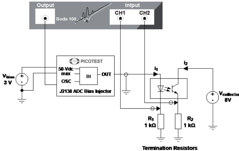
Figure 32 – Measuring an optocoupler’s maximum CTR.
