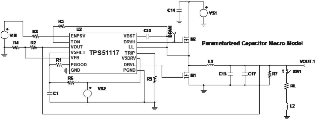
Figure 13 – Adaptive on-time transient analysis schematic.
