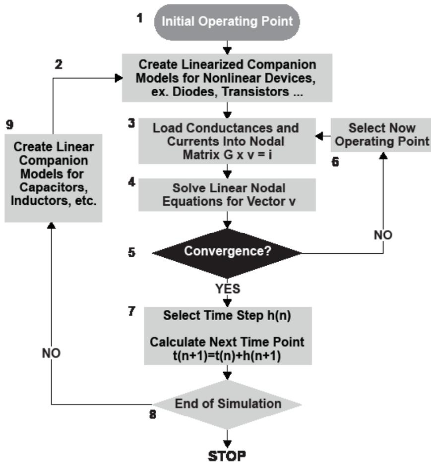
Figure 2 – SPICE basic matrix solver algorithm.
