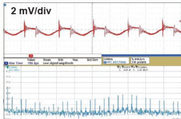
Figure 33 – High-fidelity output ripple measurements.
