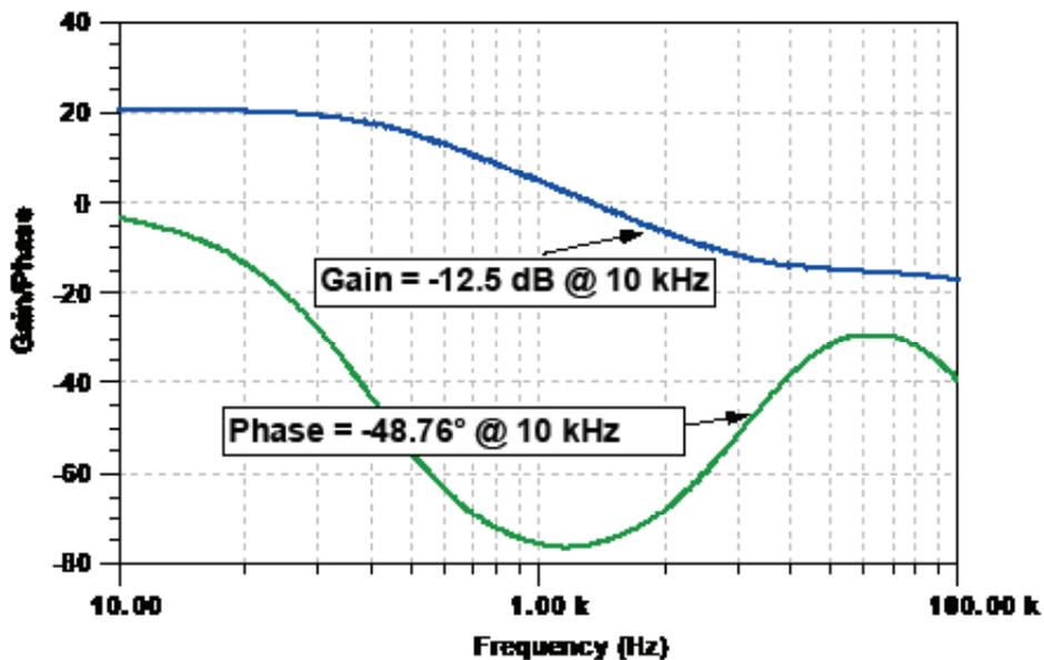
Figure 28 – Open-loop transfer function.
