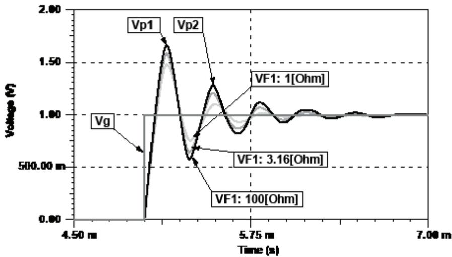
Figure 22 – Output filter time response and Q.
