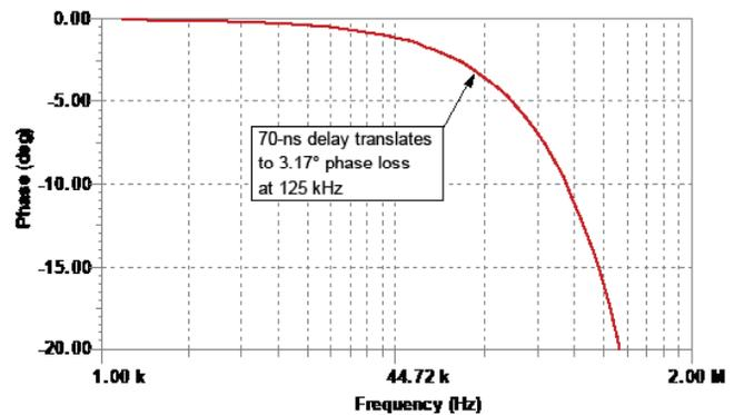
Figure 18 – Modulator delay effect on phase.
