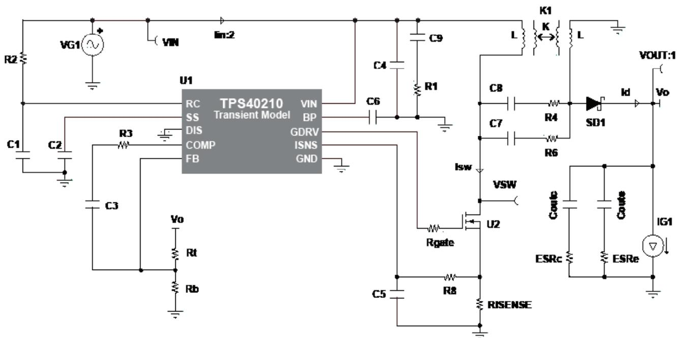
Figure 3 – SEPIC transient analysis circuit simulation model.
