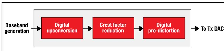
▲ The GC5322 integrates digital upconversion, crest factor reduction, and digital pre-distortion
