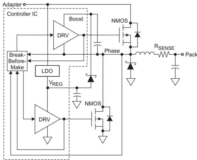
Fig. 11. Driver topology for synchronous NMOS/NMOS topology.
