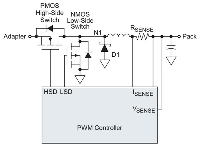
*Fig. 7. Synchronous topology with a PMOS high-side switch.*
