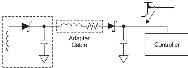
Fig. 32. Supply-line overshoot upon adapter hot-plug insertion.
