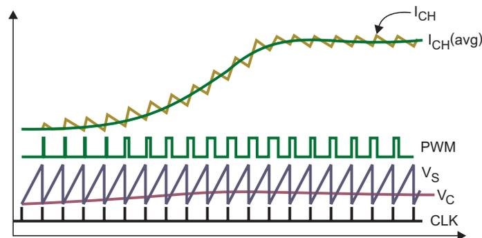
Fig. 35. Soft start ramping up the charge current.
