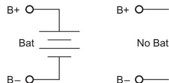
Fig. 27. Expected loads for a cradle battery charger.
