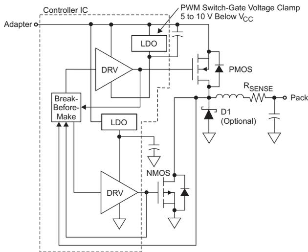
Fig. 9. Driver topology for synchronous PMOS/NMOS topology.
