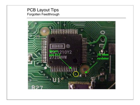
The goal was to place the resistor to protect the reset pin. The close placement of the resistor didn't solve the problem. However the feedthrough was to an external connector that defeated the purpose of the resistor.
