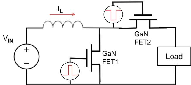
Figure 2: Boost-converter schematic
