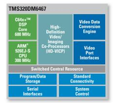
TMS320DM6467 processor block diagram
