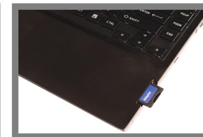
**8** To prepare your workstation for software development, power off the kit, remove the micro SD card; insert it into the included SD card adapter (if applicable); and insert it into your PC. If your PC does not include an SD slot, USB SD card adapters are readily available. Follow the instructions below.
