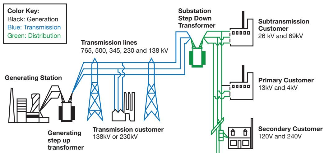
Figure 1. The Smart Grid will extend intelligence and omni-directional communications throughout the power supply system for more reliable, efficient power consumption.
