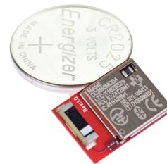
**Figure 2.** SimpleLink Bluetooth low energy CC2650MODA module
