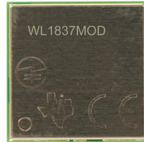
**Figure 5.** WiLink 8 combo connectivity modules for Wi-Fi and Bluetooth/Bluetooth low energy connectivity
