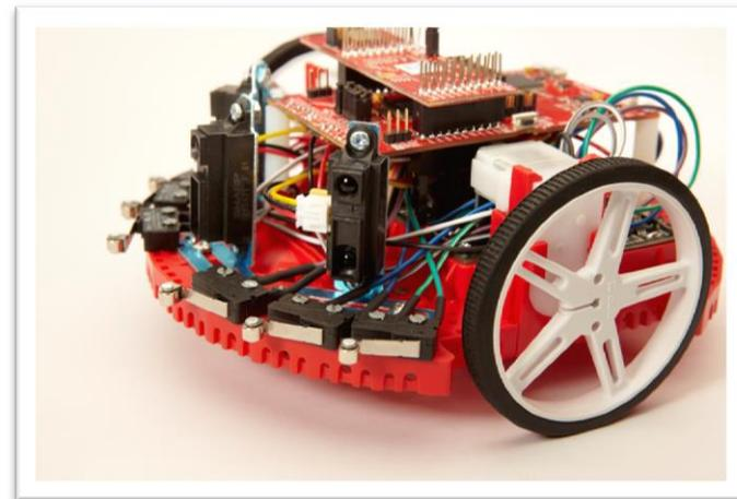
Figure 1. IR distance sensors, positioned at the front of the robot.
