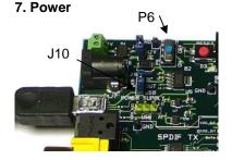
To power the PPW AudioEBs; connect a USB cable to each of the PPW AudioEBs and make sure J10 is in the position "OUT-USB" (Pos 1-2). Finally, switch P6 to "ON". The LED D3 should now be lit.
