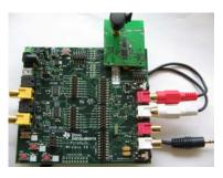
Connect an audio source (CD-player, MP3-player or similar) to the line-in input of the AudioEB with CC85xxEM or CC85xx-CC2590 with the "MASTER" label plugged in.
