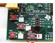
When powered for the first time, LED D9 will blink to indicate that the devices are not connected.
