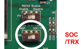
If you have a SmartRF05EB version 1.7.1 or older, it is recommended to turn off the RS232 interface for best performance.
