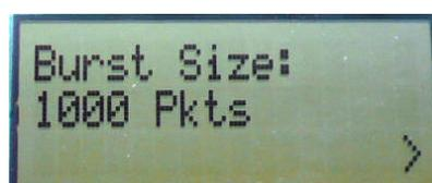
Next, select burst size (number of packets to send) by using the joystick, either 1000, 10K, 100K or 1M packets. Confirm the selection with Button 1.
