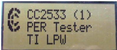
When power is applied to the SmartRF05EB, the preprogrammed PER test on the CC2533 will start running.
