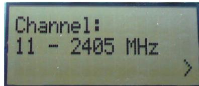
Select one of the 16 IEEE 802.15.4 channels, with channel number from 11 to 26 (2405-2480 MHz, 5 MHz channel spacing). Select the same channel for both boards.
