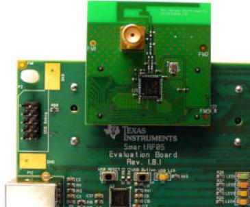
The CC2533EM can be plugged into the SmartRF05EB.
