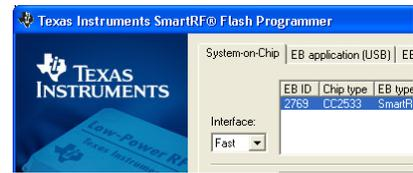
The Flash Programmer application, available on the kit web page [2], can be used to program Intel HEX files, read the contents of flash and several other operations.
