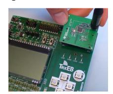
Insert a CC1120EM board into the TrxEB as shown above. Connect the antenna firmly to the SMA connector on the EM.
