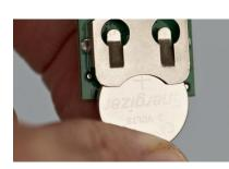
Note that when inserting the battery for the first time, the PCB contact point surface may have a thin layer of solder residue that can prevent contact with the battery. Remove and insert the battery a few times to power the SensorTag.
