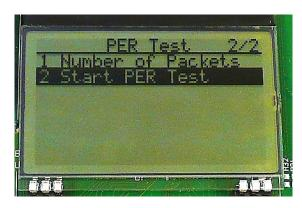
When selecting "Start PER Test", the master (receiver) will begin to count the number of received packets and provide some statistics.
