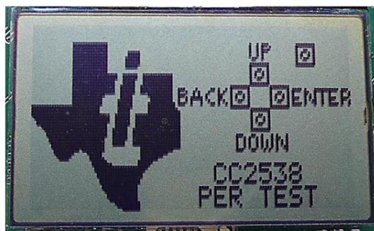
Turn on power with the Main Power switch. You should now see the Texas Instruments logo and a short description of the buttons on the LCD. Pushing any of the five buttons on the board will take you to the main menu.
