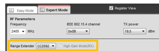
You can now configure the radio, run performance tests, export register settings and run link tests with another CC2538 on a SmartRF06EB connected to the PC.
