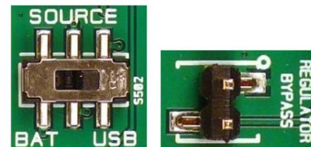
The power source is selected using the Source switch on the left hand side of the SmartRF06EB.
