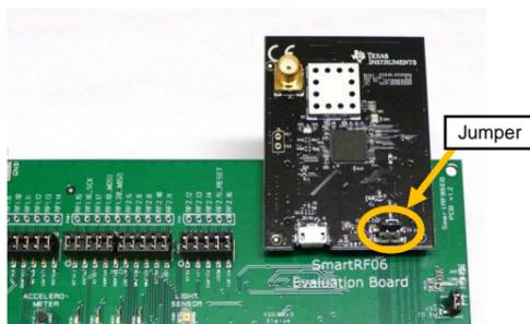
Insert a CC2538-CC2592EM board into the SmartRF06EB as shown above.
