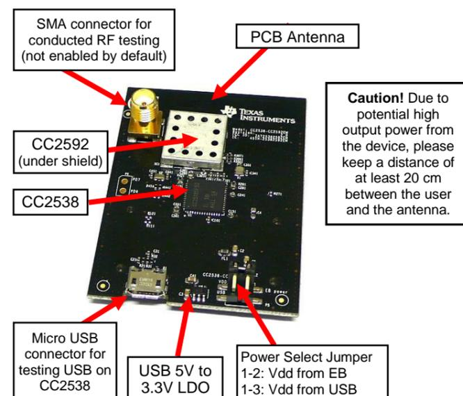
**Caution!** Due to potential high output power from the device, please keep a distance of at least 20 cm between the user and the antenna.
