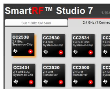
After installing the tool, connect the EB to the PC using the USB cable and start SmartRF Studio. Select the "2.4 GHz" tab and click the refresh ("Find device") button in the lower right corner. Studio will now find the connected SmartRF06EB. Double click on the detected SmartRF06EB to launch the CC2538 device control panel.
