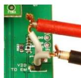
It is also recommended to isolate the EM from the SmartRF06EB by removing the breakout jumpers and XDS100v3 bypass jumpers.
