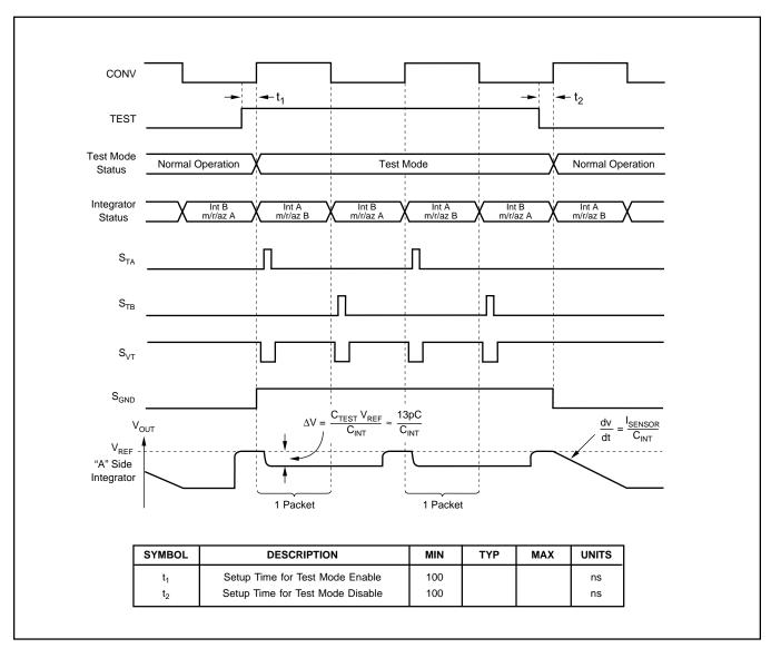
FIGURE 2. Single Packet Test Mode Timing.
