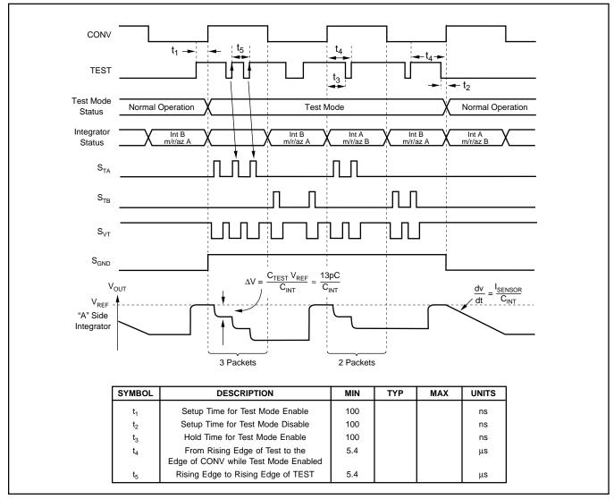
FIGURE 3. Multiple Packet Test Mode Timing.
