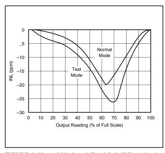
FIGURE 4. Normal Mode and Test Mode INL (end-point line fit).
