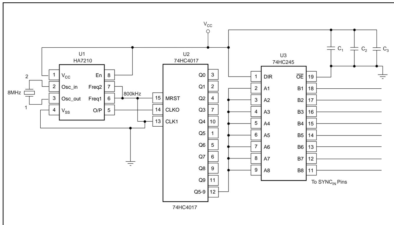
FIGURE 9. Crystal-Generated Clock Signal.
