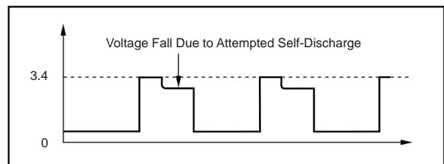
FIGURE 5. 74HC245 O/P Drive Waveform.
