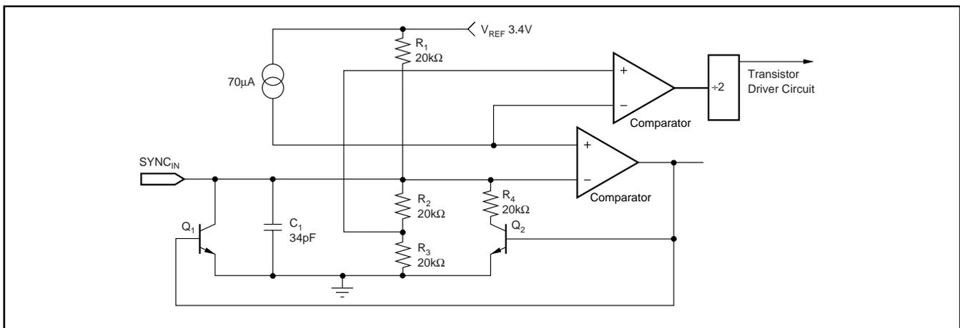
FIGURE 2. Internal Oscillator Circuit.
