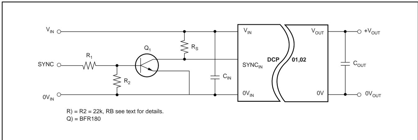
FIGURE 11. External Control of the DCP01, 02.
