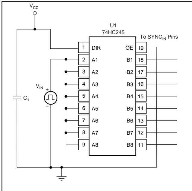
FIGURE 6. DCP01 Series HCMOS Interface.
