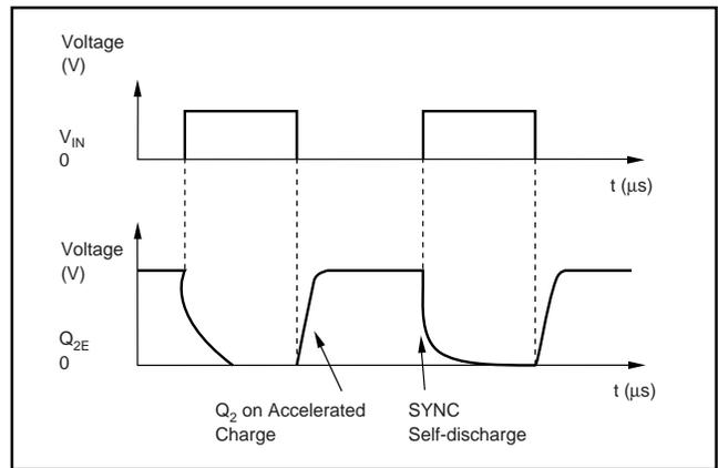
FIGURE 4. Emitter Follower Output Waveform  $V_S$  and  $V_{IN}$ .
