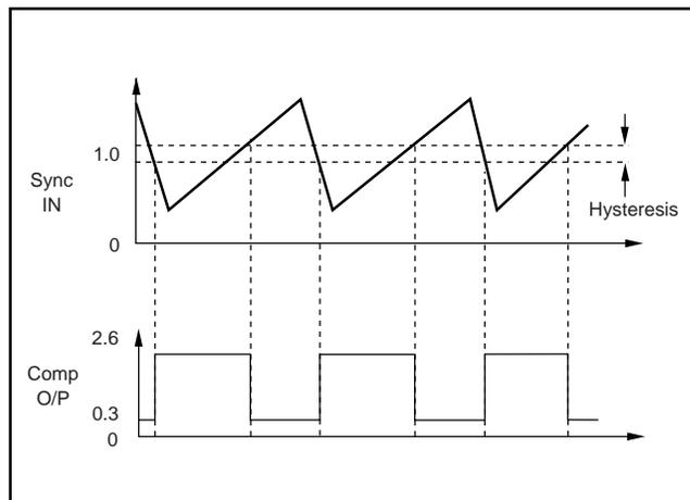
FIGURE 8. Comparator-Generated Timing Pulses.
