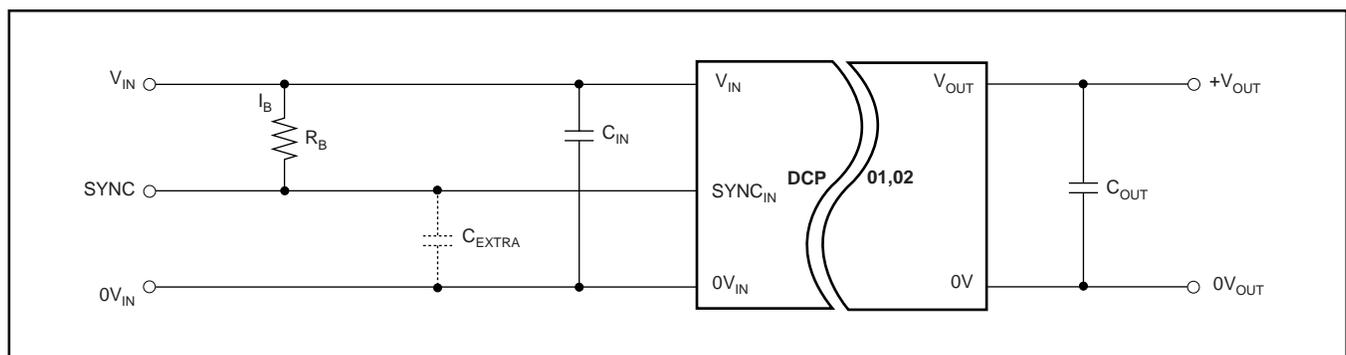
FIGURE 10. Connecting a Bleed Resistor.
