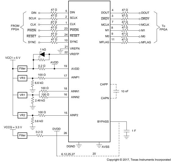
Figure 11. Test Circuit
