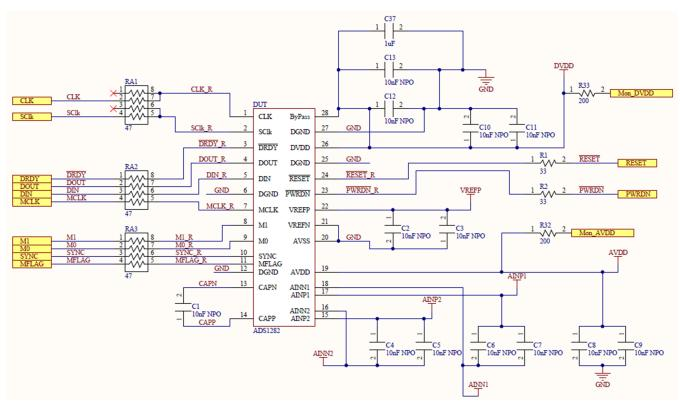
Figure 6. DUT Schematic, DVDD < 2.25 V
