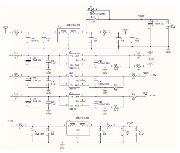
Figure 7. Input Power Circuit
