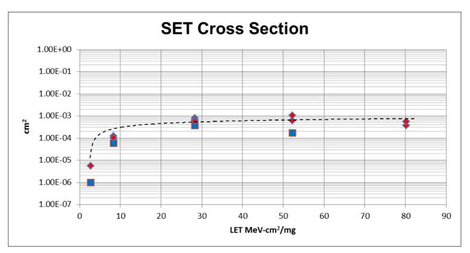
Figure 15. SET Cross Section
