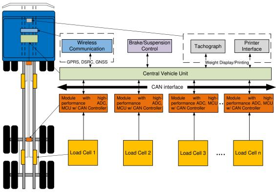
Figure 1. Typical Implementation of an On-Board Weighing (OBW) System
