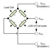
Figure 2. Typical Load-cell Implementation
