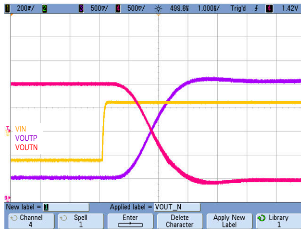
Figure 8-4. Step Response of the AMC1301
