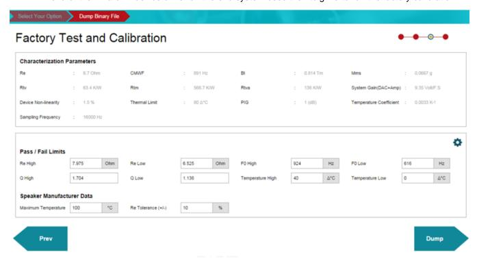
Figure 8. Factory Test and Calibration
