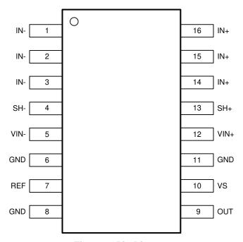
Figure 2. Pin Diagram
