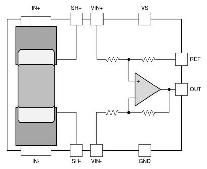
Figure 1. Functional Block Diagram
