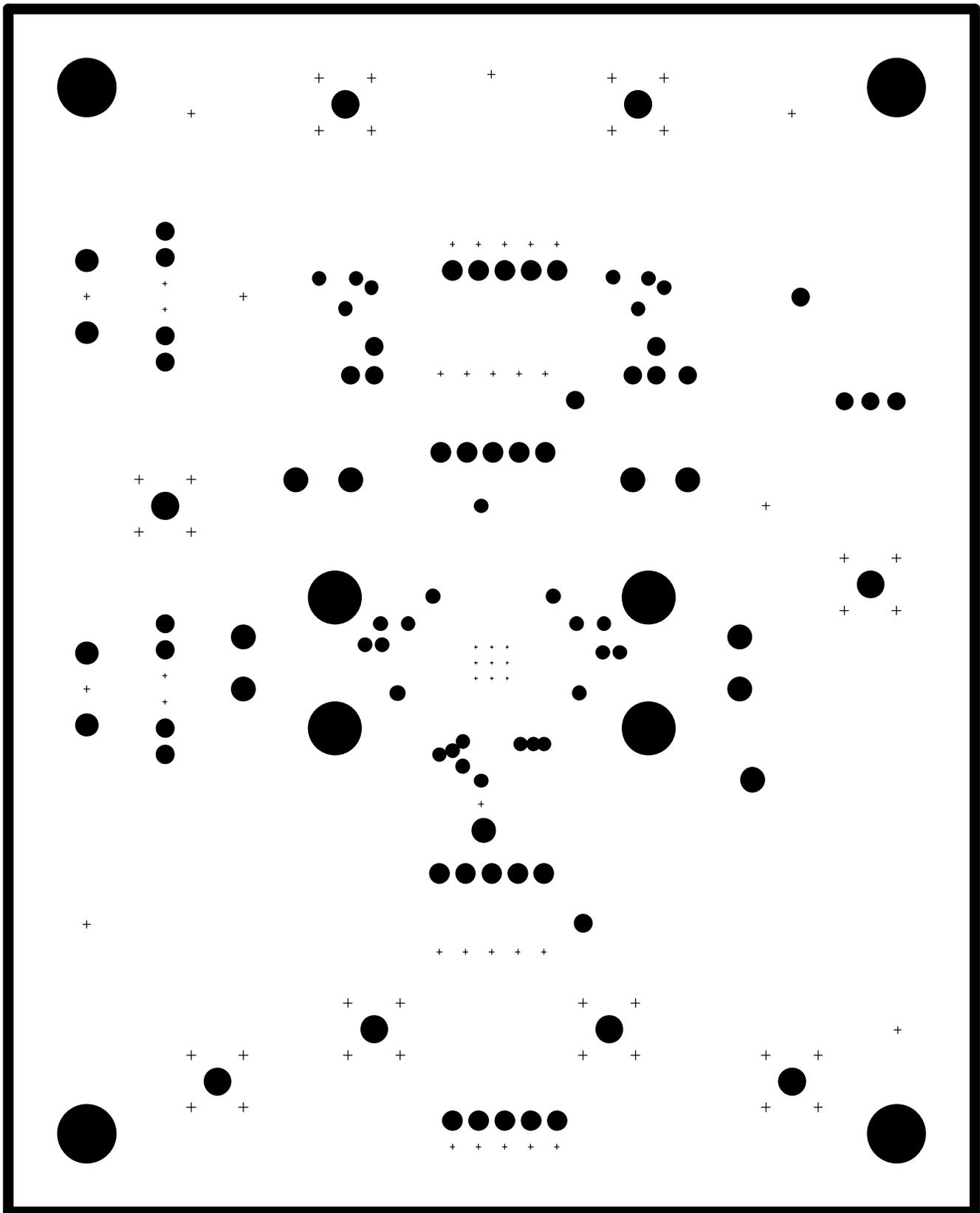
Figure 4. VCA2615EVM PCB Ground Layer (Top View)
