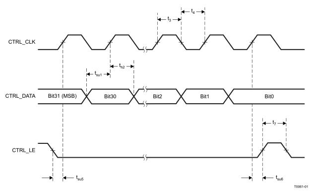
Figure 1. Timing Diagram SPI Control Interface
