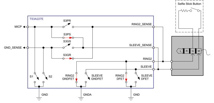
Figure 5. TS3A227E Switch State After Detecting a 4-Pole OMTP Headset
