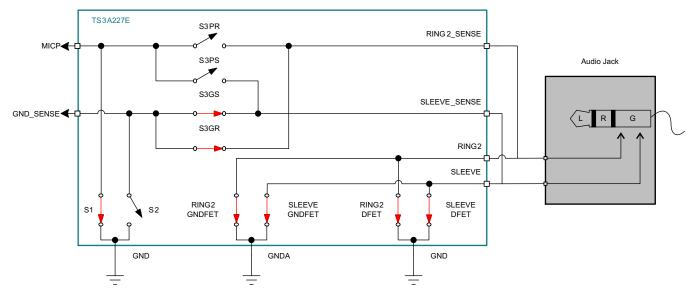
Figure 14. TS3A227E Switch State After Detecting a 3-Pole Headphone
