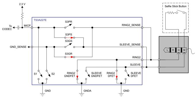
Figure 9. Microphone Bias is High With Selfie Stick Inserted Into the Audio Jack Receptacle
