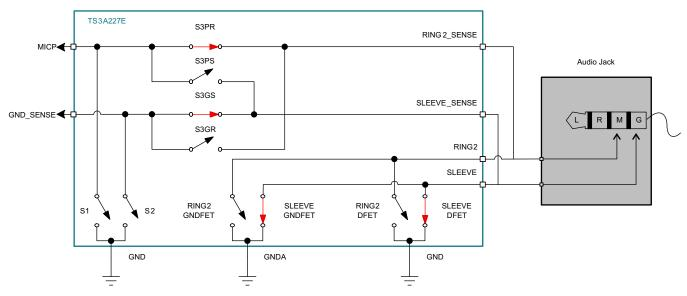
Figure 15. TS3A227E Switch State After Detecting a 4-Pole OMTP Headset
