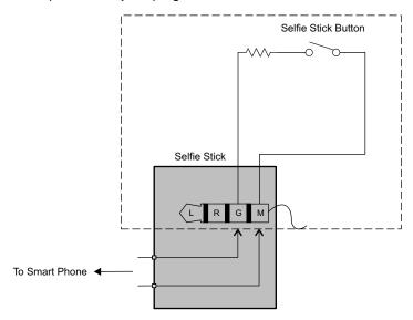
Figure 1. Typical Selfie Stick Schematic
