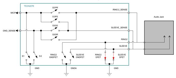
Figure 12. TS3A227E Default Switch State With no Accessory Inserted
