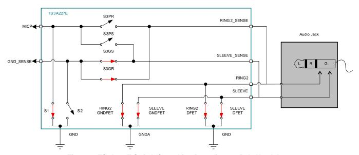
Figure 7. TS3A227E Switch State After Detecting a 3-Pole Headphone
