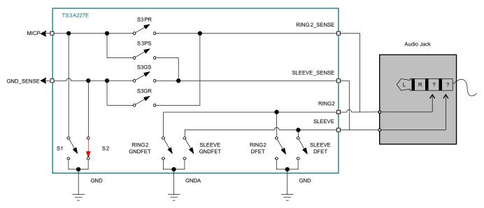
Figure 13. TS3A227E Switch State During Detection
