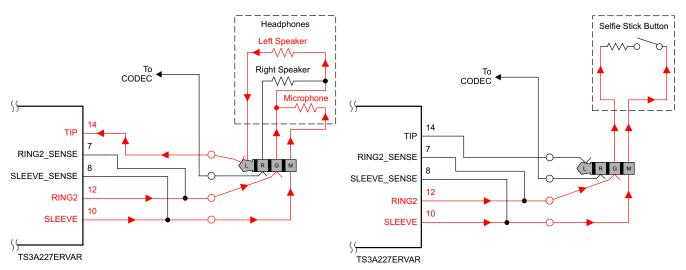
Figure 2. TS3A227E Application Circuit With Closed Circuit From Ring2 To Tip Made With Headphone Accessory
