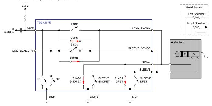
Figure 10. Microphone Bias is Low With 3-pole Headphones Inserted Into the Audio Jack Receptacle
