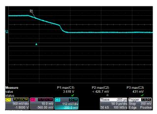
Figure 6. DRL Power down testing
