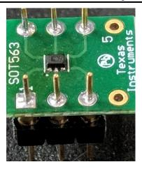
Figure 4. Soldered SN74AXC1T45DRL With Header Pins
