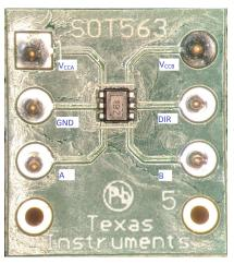
Figure 3. Soldered SN74AXC1T45DRL (Microscope Image)
