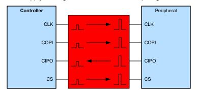
Figure 2-1. SPI Translation for System Controller to Wi-Fi<sup>™</sup> Module Interface
