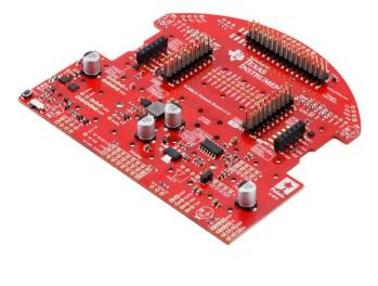
Figure 1. TI-RSLK Chassis board (www.pololu.com).
