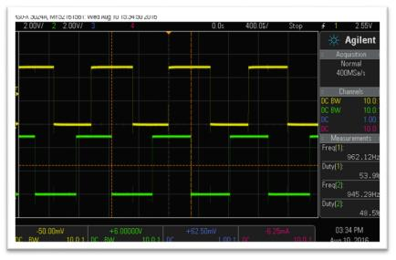
Figure 1. Scope trace of the two outputs of the tachometer, period\*360 is the time for one revolution. (From https://www.pololu.com/product/3542/)
