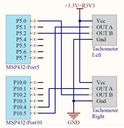
Figure 1. TI-RSLK chassis board connecting the encoders to the MSP432.
